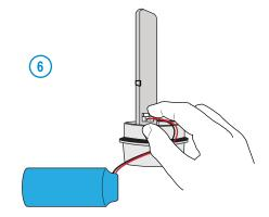
Plug the new battery cable into the circuit board.
