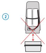
Do not disconnect the circuit board from the radar.
