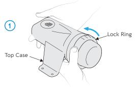
Unscrew the lock ring anti-clockwise. The circuit board, battery and radar can now be removed from the top case.
