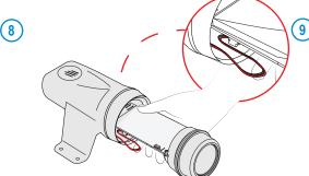
Slide the circuit board and radar into the new case over the battery. Push the case and radar together to compress the
